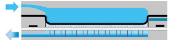
FIGURE 5. The second squeeze with the pressing diaphragm forces the wash water to pass through the cake in a uniform front.
