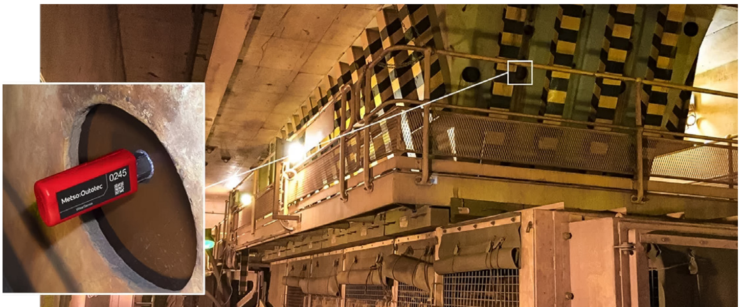
Wear sensor installed in a coarse ore stockpile
