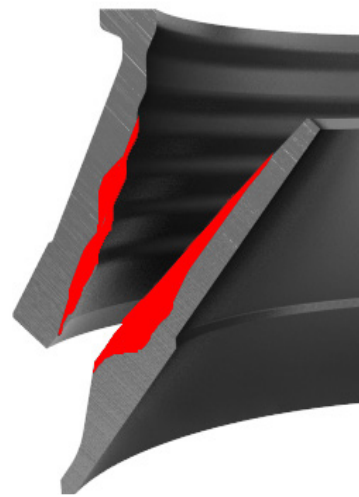
Example of abnormal wear. Cupping has occurred.
