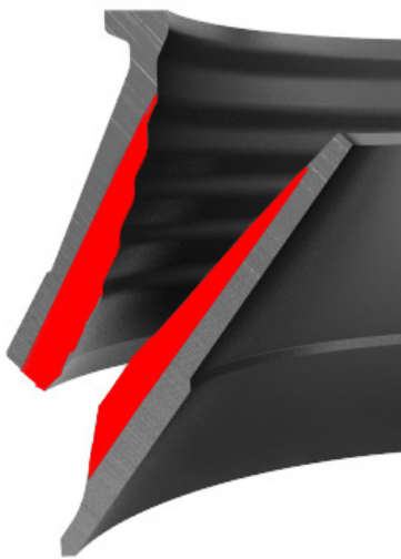
Example of normal wear. Obtained with correct feed arrangements, feed gradation and parameters for the chamber.
