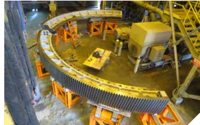
A 40,000 lbs gear segment being prepared for reversal
