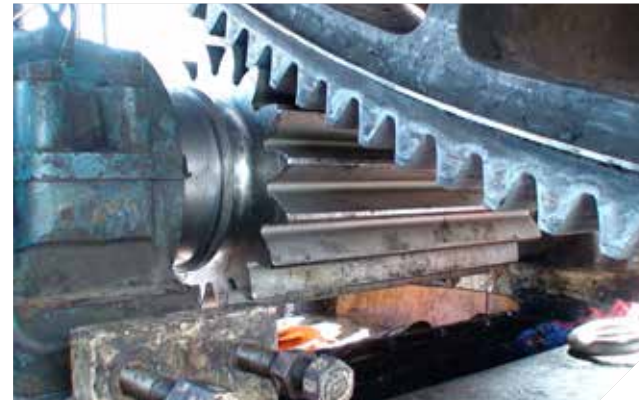
Pinion being aligned to the reversed gear
