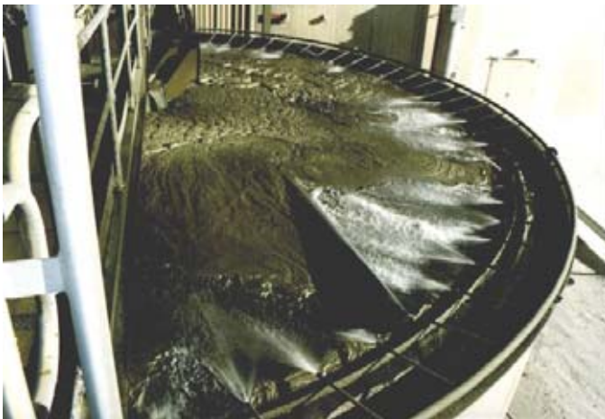
Froth baffle & peripheral sprays
