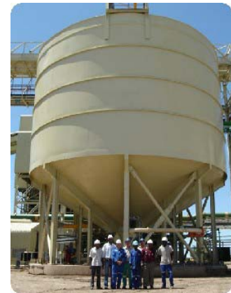
Paste thickener – very deep sidewall, increased floor cone angle
