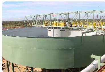
High compression thickener – increased sidewall depth
