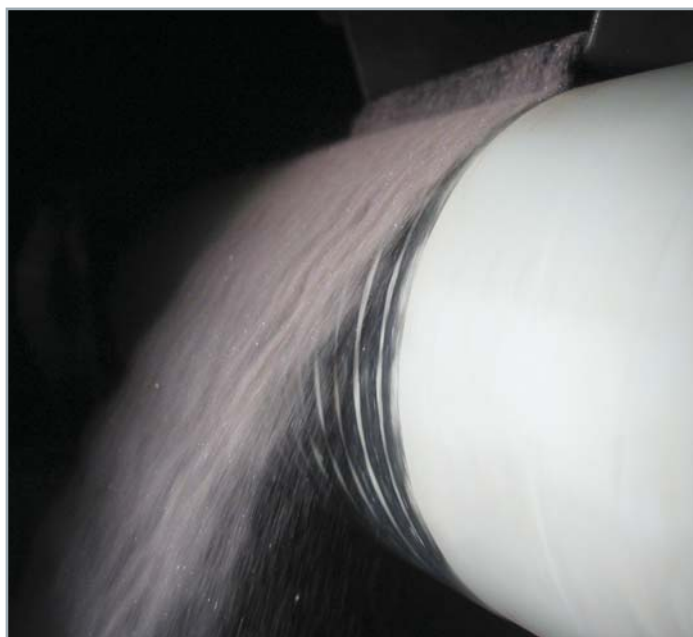
To combat this increase in fines, companies are advancing traditional technologies like advanced rare-earth roll separators that are more suited for materials <math><75\mu\text{m}</math>.
