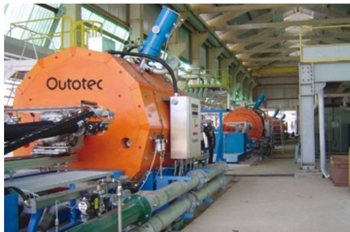
Cryofilter® HGMS systems treating a sedimentary kaolin deposit
