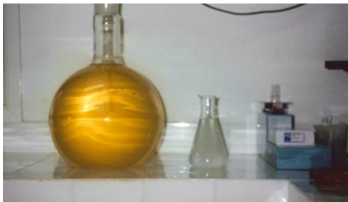
Two examples of problematic water supplies. Left: process water with obvious color staining. Right: process water with not so obvious suspended particulates.
