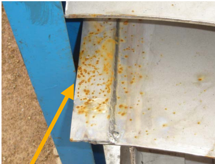
Cross contamination from nearby grinding which has lead to rust formation on stainless steel
