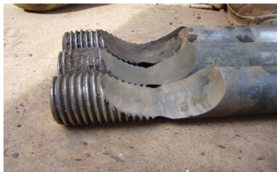
Studs damaged through slurry racing
