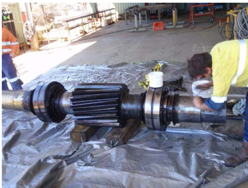
Stripping and rebuilding a spare pinion
