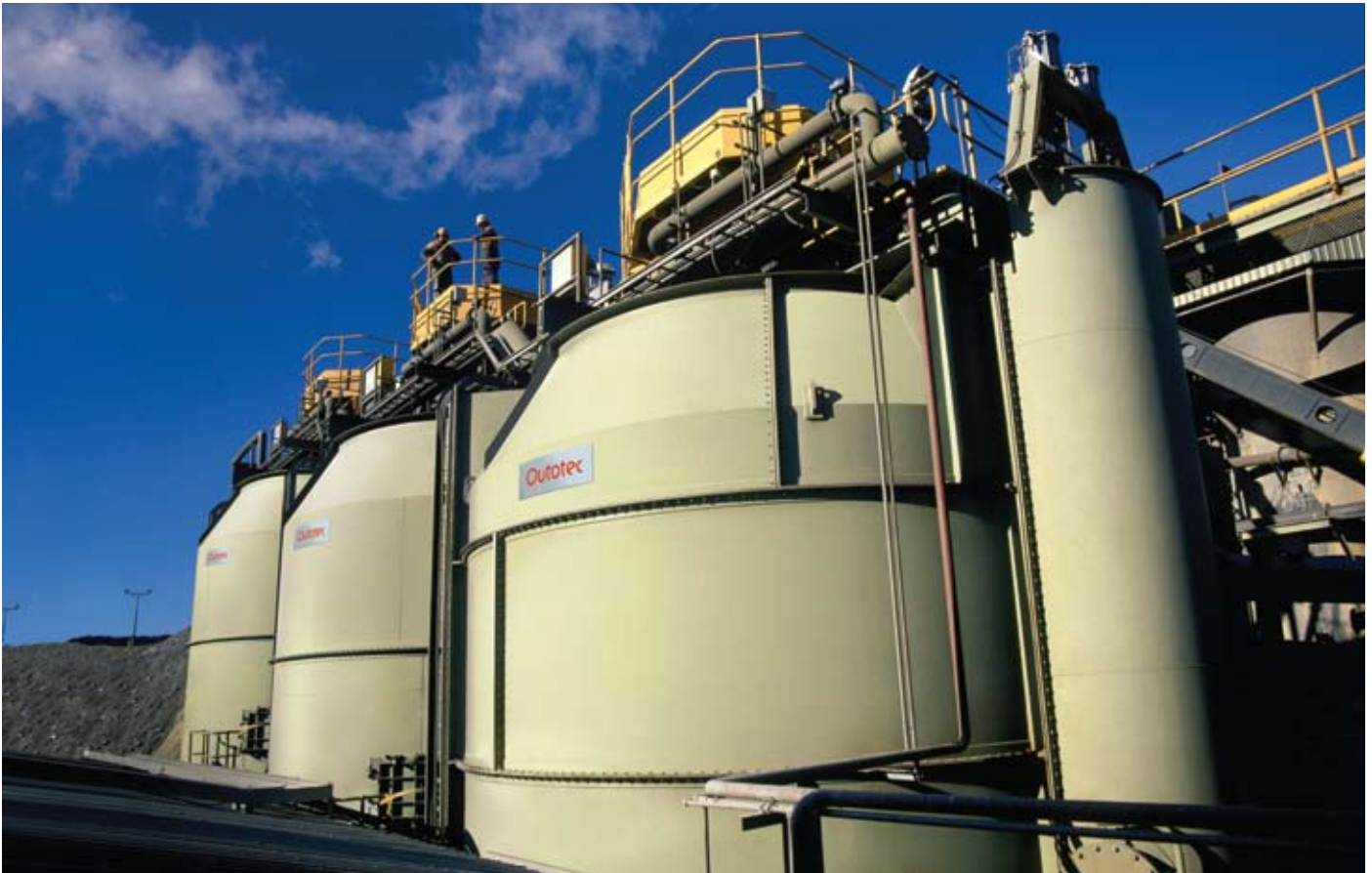
The 3 x TankCell® -300 at Macraes. The world's largest operational flotation cells, with over 300m 3 active capacity.
