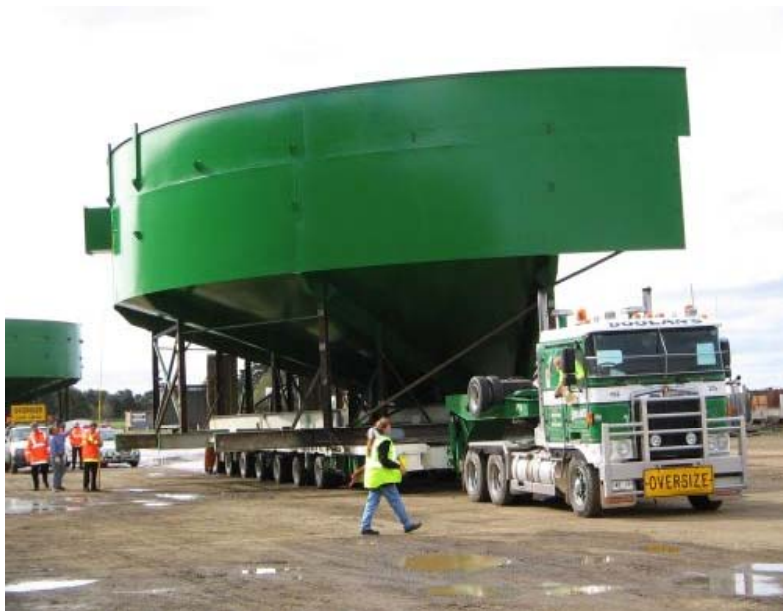
Transportation of piece large thickener tank
