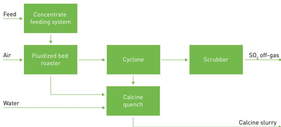
Sulfating roasting is generally used for processing copper concentrates in combination with electrowinning. The copper sulfide is transformed into water-soluble copper sulfate and the iron sulfide into insoluble iron oxide. Standard sulfating roasters run with a slurry feed and do not require a waste-heat boiler system in the off-gas stream.
