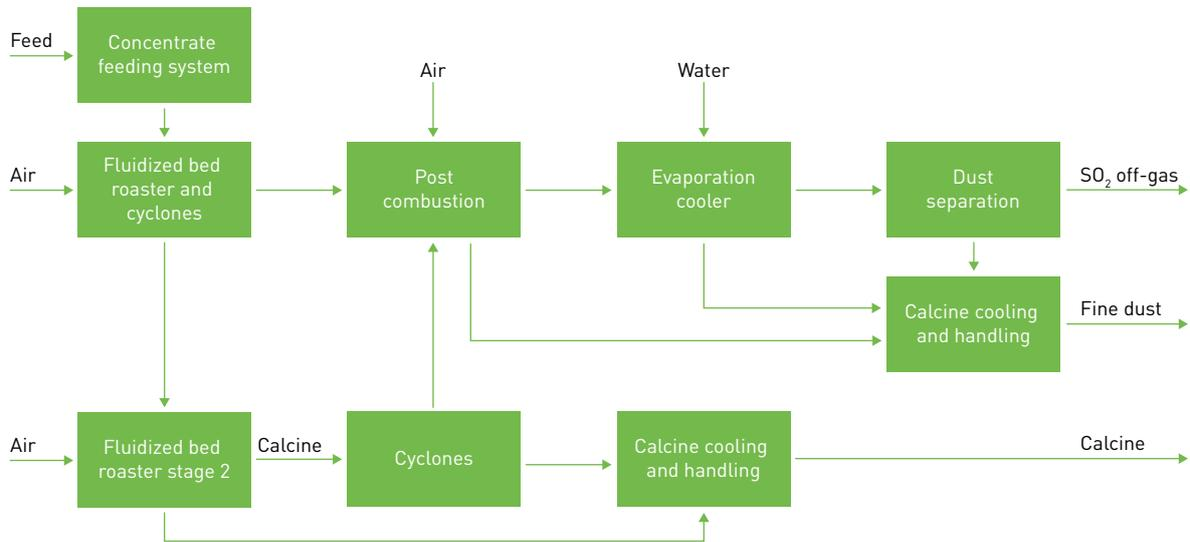
Our two-stage roasting plants are mainly used for treating double-refractory gold concentrates. A two-stage roasting process combines partial roasting in the first stage with dead roasting in the second stage. The first stage is used as a de-arsenifying process step in an oxygen-deficient roasting atmosphere, while the second stage operates in an oxidizing atmosphere to fully transform the metals into their oxide form.
