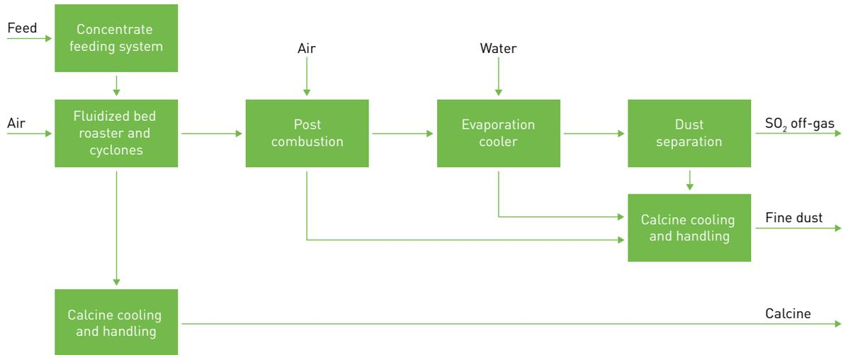
Our partial roasting process is used for removing impurities from feed material. In this process the sulfur is only partially roasted, with the quantity depending on the concentrate analysis and the desired calcine grade. In some cases, partial roasting is used to remove almost all unwanted elements – such as arsenic and antimony – before further treating the calcine. Special equipment is used for cooling and precipitating arsenic trioxide, which can be produced to a very high purity.
