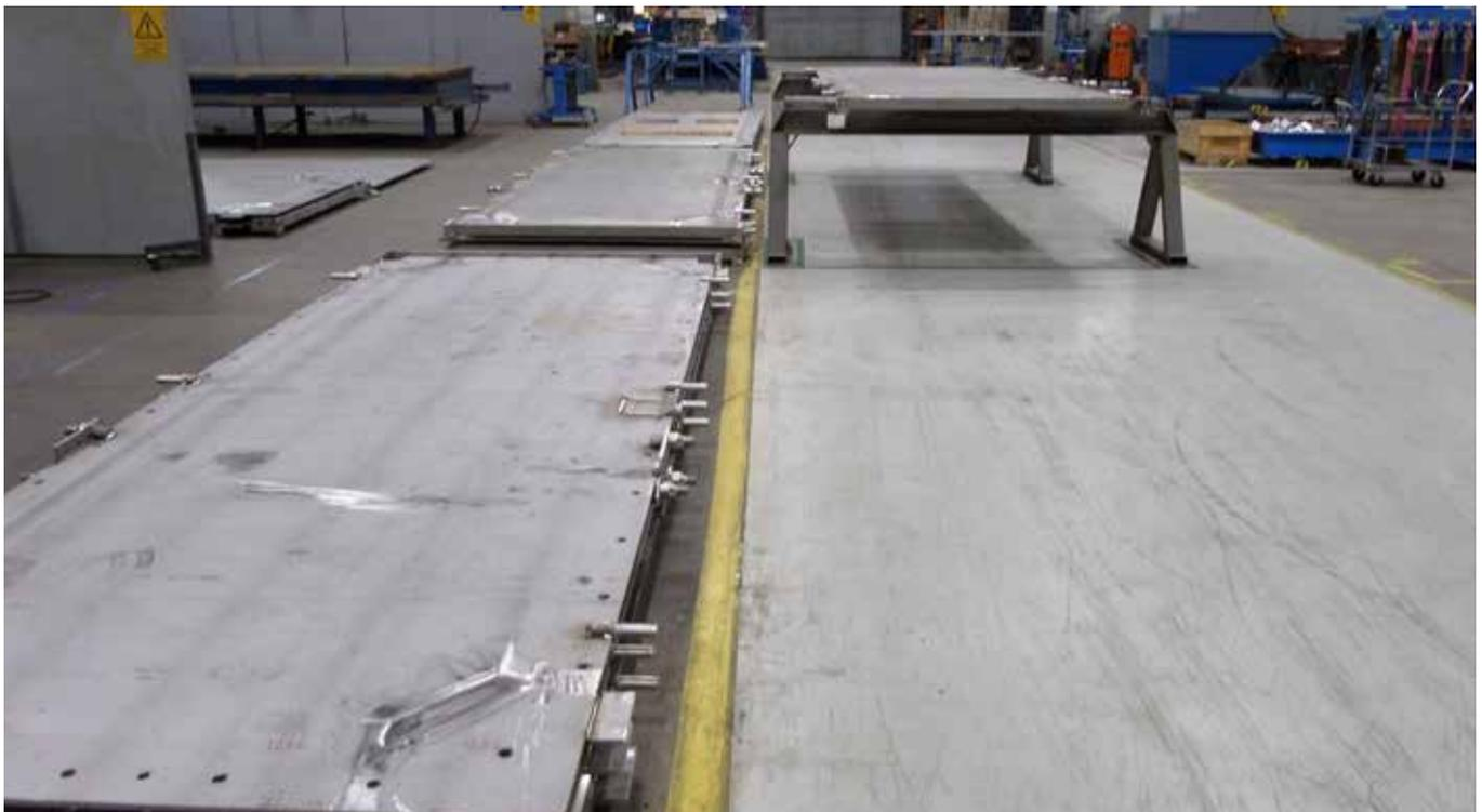
Plate under manufacture prior to weld out.
