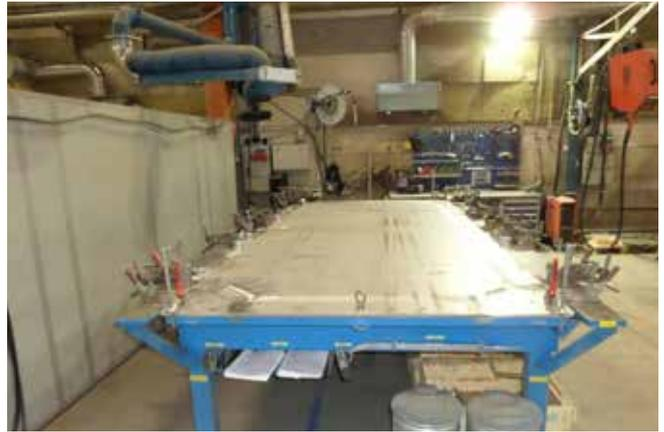
**Plate mounted in jig for weld sequencing and distortion control.**
