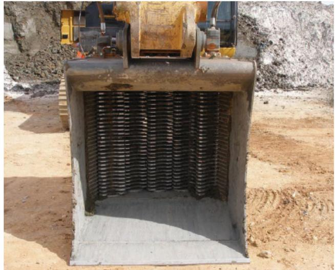
MISU unit fitted to an excavator
