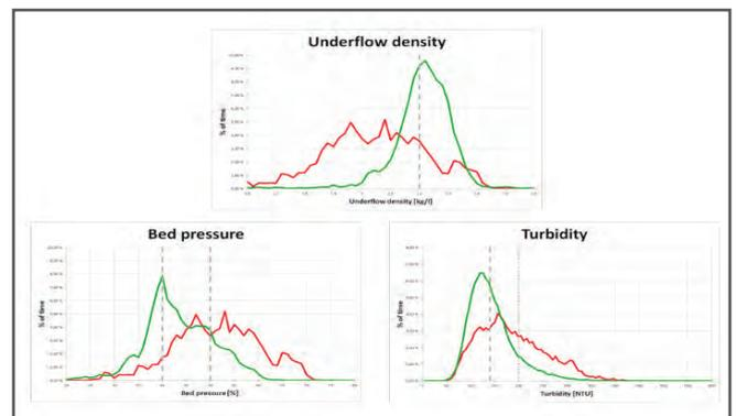
**Relative distribution of underflow density, bed pressure and overflow turbidity - manual control (red curve) vs. thickener optimizer (green curve)**
