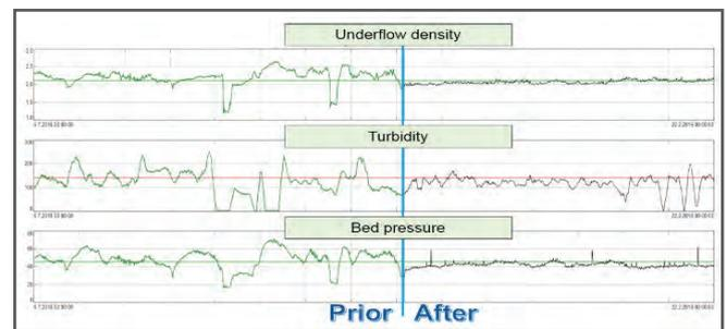
**Thickening performance - manual control vs thickener optimizer**
