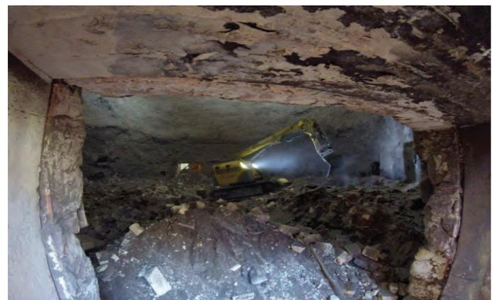
Safe, remote cleaning and removal of rubble from roaster nozzle grate
