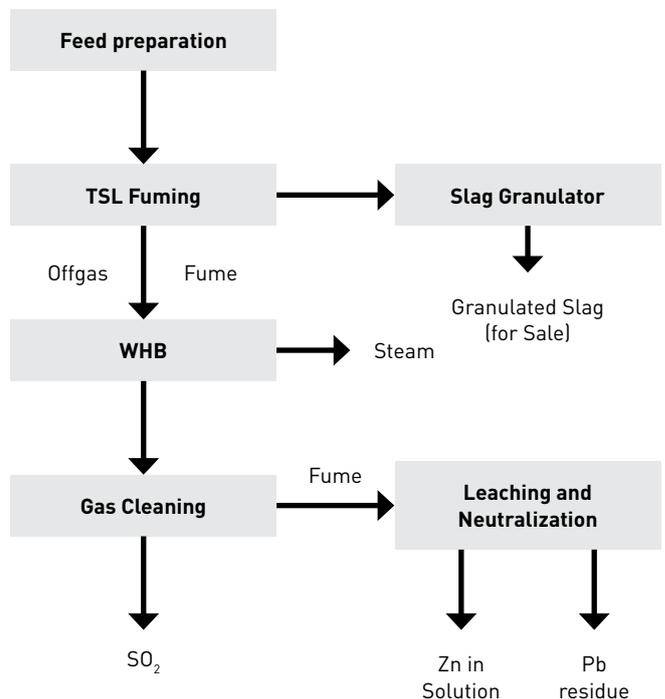
World zinc production has been steadily increasing by 4% per annum to 13 million tons in 2012. The majority of this zinc production is produced via the Roast-Leach-Electrowinning (RLE) process, which eliminates iron from the circuit in the form of leach residues such as goethite, paragoethite or jarosite. For every ton of zinc metal produced using the RLE process, usually 0.5 to 0.9 tons of zinc residues is generated.
