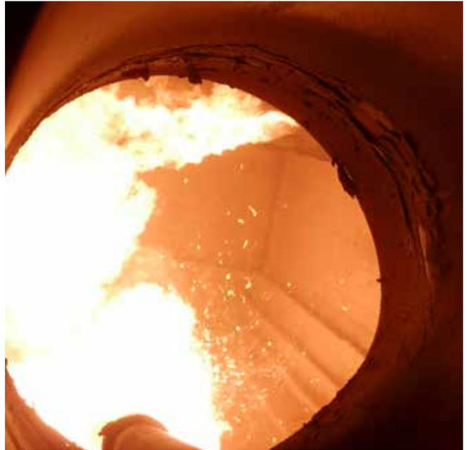
Initially the matte grade produced was 62% Cu in order to achieve a high heat value for the feed mixture for the start-up of the Flash Converting Furnace. The feed rate in the beginning was 80 t/h and increased gradually to 150 t/h once the concentrate conveyors and -dryers were capable of supplying more concentrate. Also the matte grade was increased to 64% Cu.
