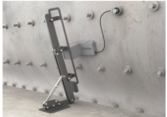
Outotec MillSense provides on-line analysis of the mill charge position and volume.
