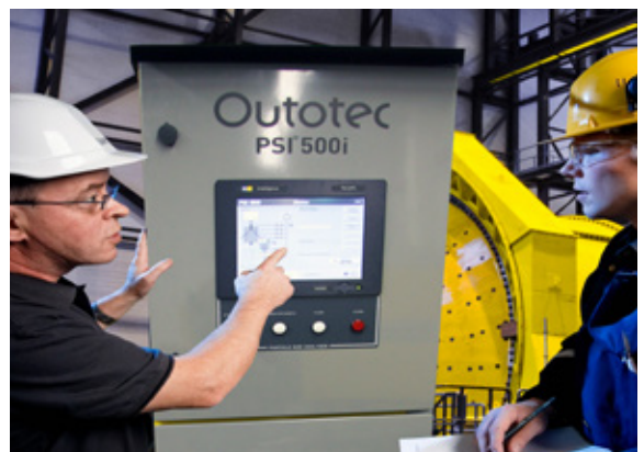
The Outotec PSI particle size analyzer is an on-line sizing system for mineral slurries.
