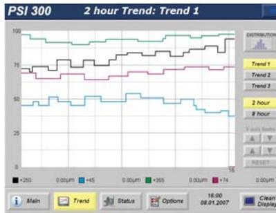
Each of the three trend displays shows four configurable size fraction trends plotted either on a 2-hour or 8-hour time scale.
