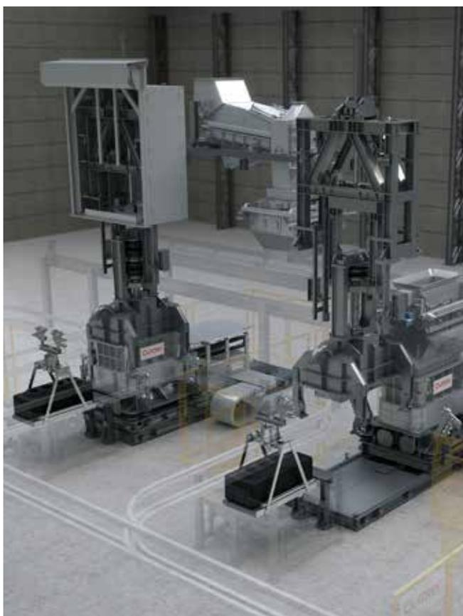
One of the two tandem anode vibrating compactors
