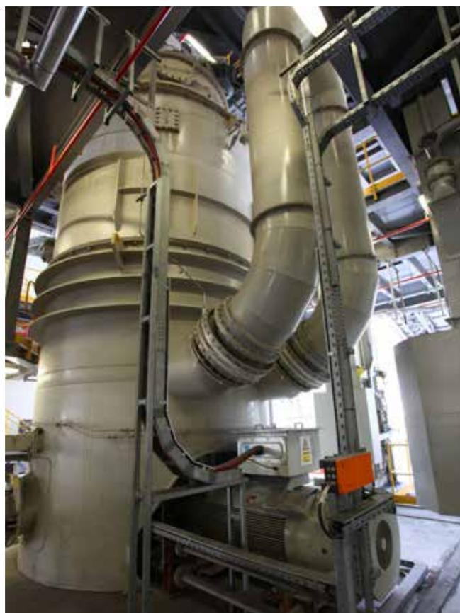
Vertical mill for coke grinding
