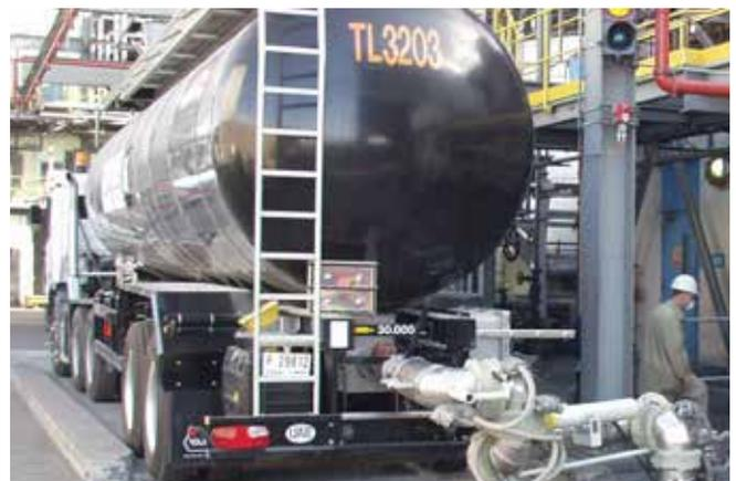
Unloading road tankers using hydraulically actuated unloading arm with quick-connection coupling for easy operation.
