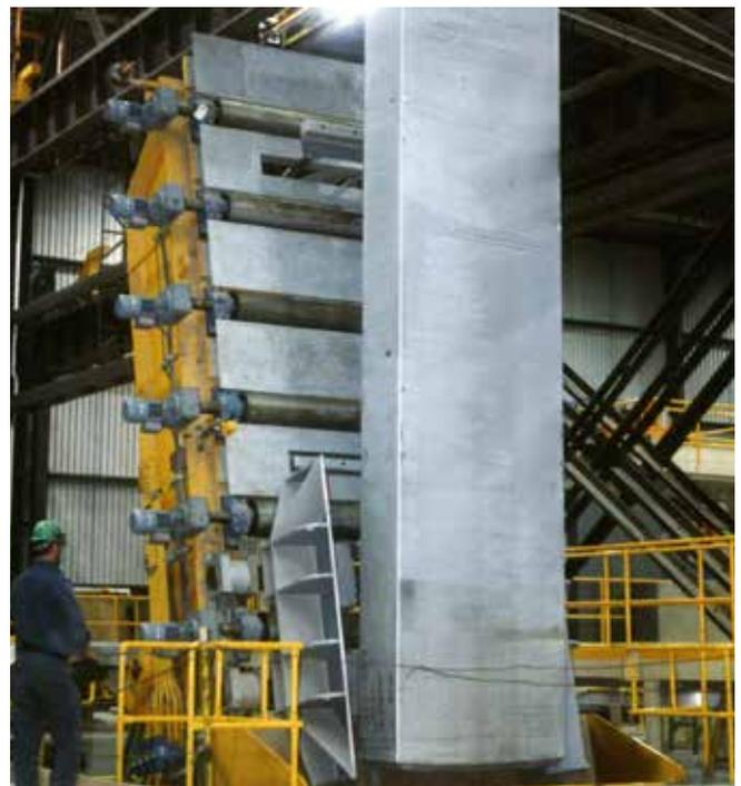
Rolling slab saw and handling.
