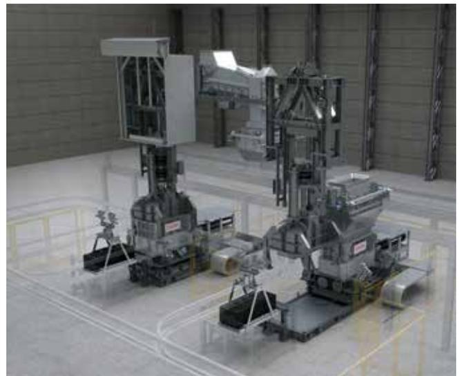
Outotec vibrating compactors ensure production of high-quality green anodes for modern aluminum smelters.
