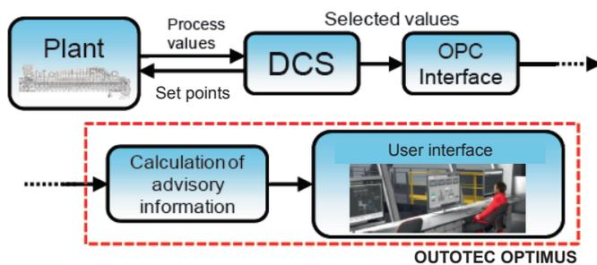
**FIGURE 3:** Structure of Outotec Optimus and integration into the plant control system
