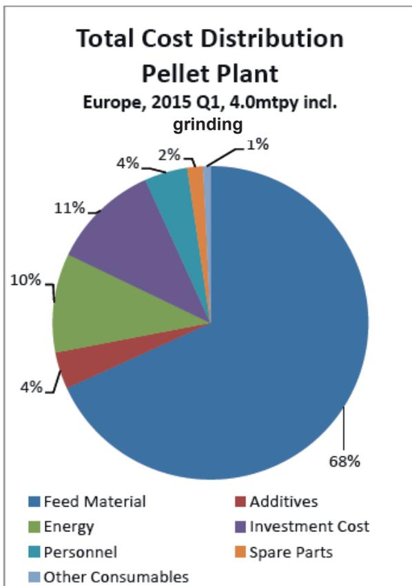
**FIGURE 1:** Breakdown of operational costs for a pelletizing plant
