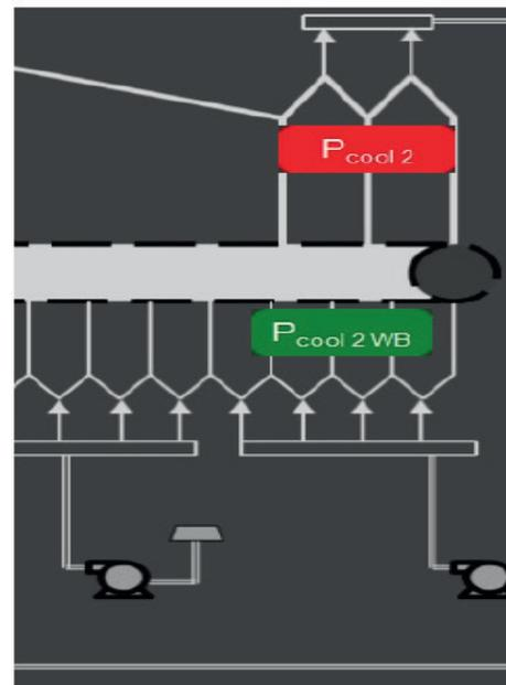
**FIGURE 4:** Outotec Optimus indicating that the operator should take steps to address an issue in the final cooling zone
