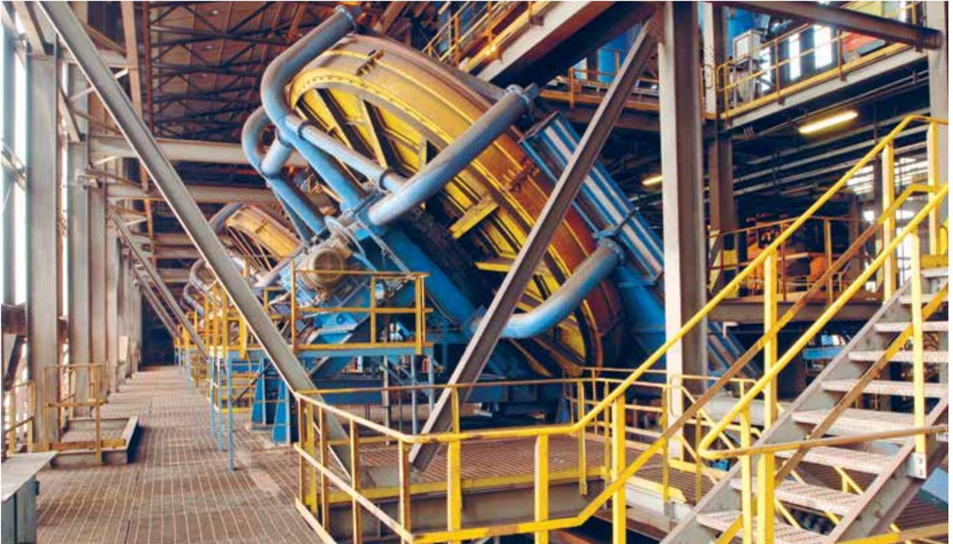
The Outotec Traveling Grate Pelletizing process consists of a green balling section where, after the mixing stage, green pellets are formed either by rolling on discs or in drums. The green pellets are then screened and heat-hardened in the indurating furnace.
