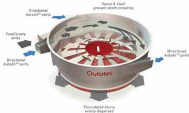
The upper zone, into which feed, dilution water and flocculant are added, provides enhanced mixing and energy dissipation. This maximizes flocculant adsorption, eliminates the possibility of coarse/fines segregation and ensures all particles are aggregated together by the flocculant. Efficient operation is maintained in this upper zone over varying feed rates.
