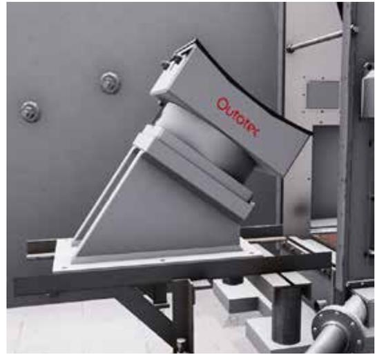
damage a conventional bronze or white metal bearing. The Outotec Polymer HSB system eliminates the requirement for emergency oil lubrication systems, such as accumulators, and requires less bearing oil flow, thereby reducing operating costs. The result is a bearing system which virtually eliminates unplanned shutdowns due to bearing failures (or emergency oil delivery system failure), thereby maximizing mill availability.
