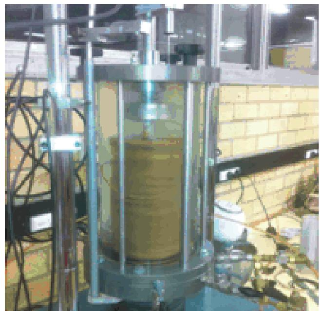
Consolidated undrained triaxial testing of Wambo paste.
