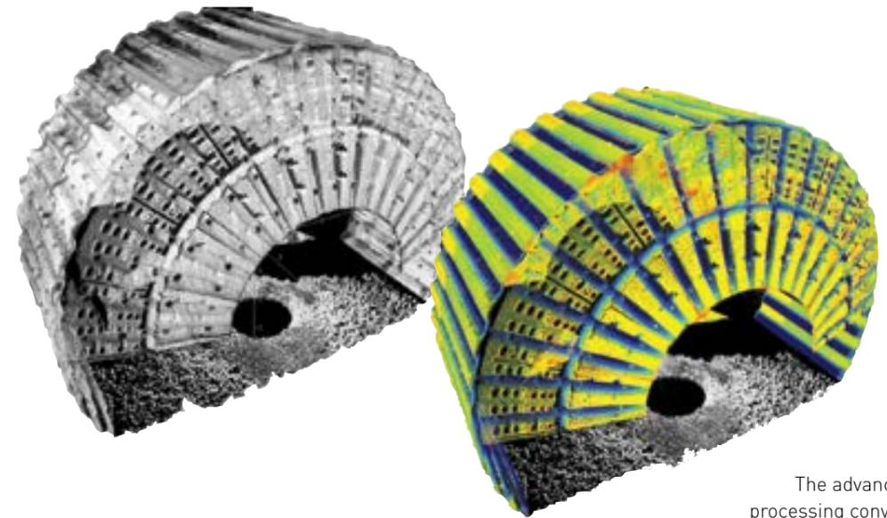
The advanced data processing converts the grey-scale surface model to a 3D liner thickness model
