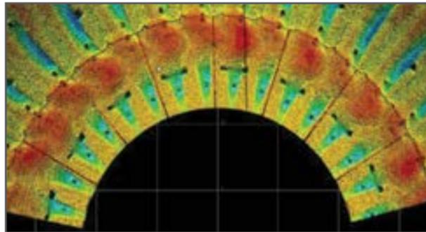
Feed end of SAG mill showing extreme wear patterns on Inner liner
